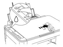
The unit begins charging the ink delivery system. This process takes about one minute to complete. When the ink charging process is finished, The On light stops flashing and remains lit, and the Ink light goes out.
