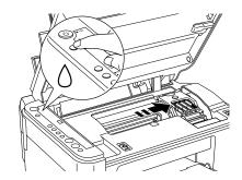
5. For best results, shake the ink cartridge four or five times before opening the package.
