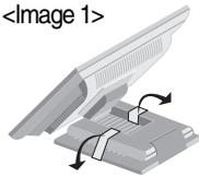
Put the set as the picture below <Image 1> to remove the tape.
