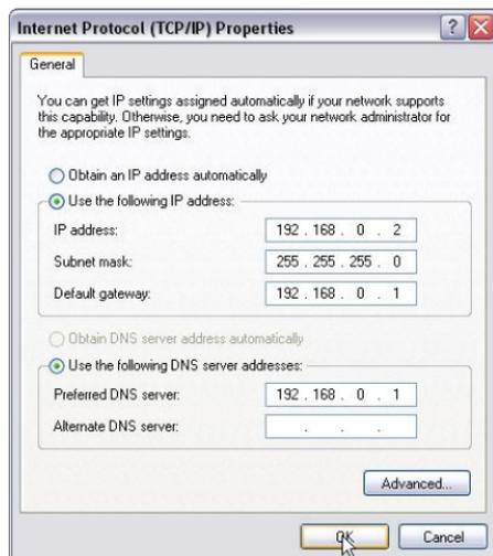
Tip: If you are not sure of the DNS server address, we recommend you to select “Obtain an IP address automatically (O)” and “Obtain a DNS server address automatically”.
