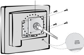
Kensington Security Slot- optional Connected to a locking cable that can be purchased separately at most computer stores
